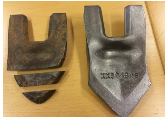
Figure 11 – Dimensional differences between a worn and new (tine) point.
