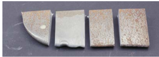
Figure 5 – Worn piece from the BOE of a loader bucket.
