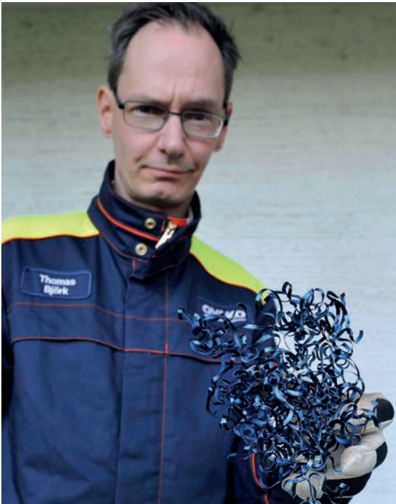
Figure 3 – Long chips can tangle around the workpiece causing tool damage and health and safety issues.
