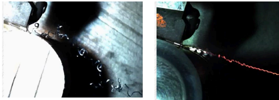
Figure 5 –Using M-Steel in hard part turning can result in chips glowing with heat as shown in the photograph on the right.
