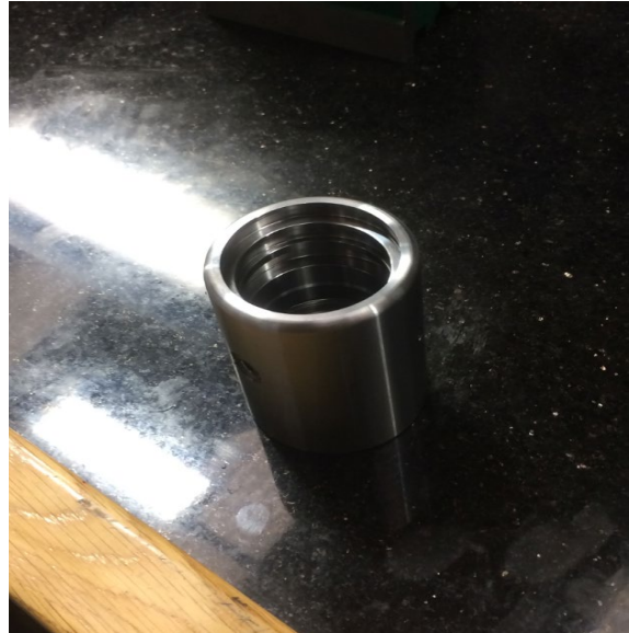
Figure 16 – PB Tech has achieved an 8% reduction in cycle time by manufacturing bushings for hydraulic components in M-Steel.
