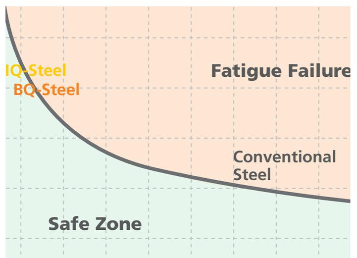
BQ-Steel and IQ-Steel have significantly smaller inclusion sizes compared to conventional steel. Note how the curve in the upper-left-hand corner is much steeper, meaning that the gain in fatigue strength is increasing exponentially.
