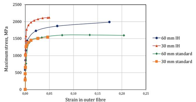
Fig 2: Stress-strain curves in 3-point bending comparing hardened and non-hardened hard-chrome plated piston-rod material (base steel 280X).
