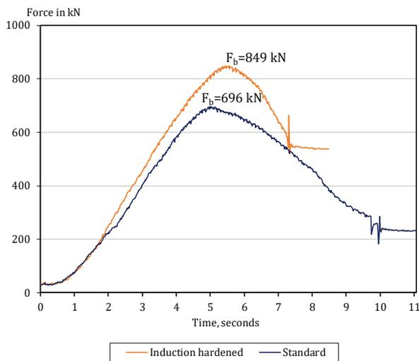
Fig 4: Comparison of force-time curves in buckling tests on hard-chrome plated non-hardened and induction-hardened piston rods (grade 280X).
