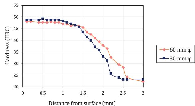
Fig 3: Hardness distribution in induction-hardened, hard-chrome plated rods giving the 3-point bending data in Fig. 2 (base steel grade 280X).
