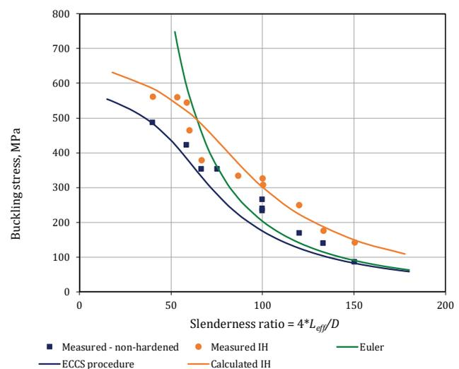
Fig 5: Buckling diagram showing measured data for non-hardened and induction-hardened chrome-plated piston rods (grade 280X) and curves calculated as described in the text.
