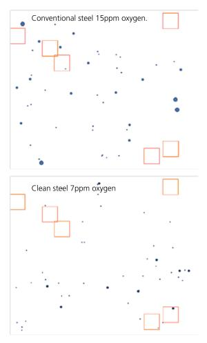
Fig 4 – A specific issue with LOM is the small sample size as shown in this schematic illustration (not to scale). Normal procedure is to examine 6 samples. But their small size does not represent the true size and distribution of inclusions. In this particular case it is even possible to obtain the false impression that standard steel (4a) has fewer and smaller inclusions than a clean steel (4b).
