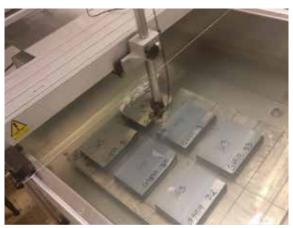
Fig 6 – immersed ultrasonic testing at Ovako
