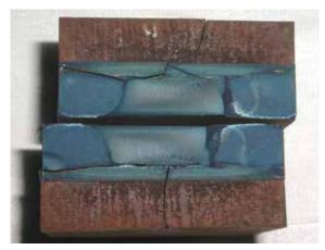
*Fig 8 – Blue fracture test showing no indication of any inclusion*
