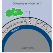
Barrier protection of the inner nickel layer
