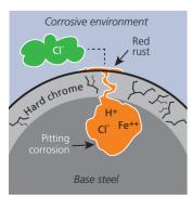
Corrosion mechanism of hard chrome plated bar
