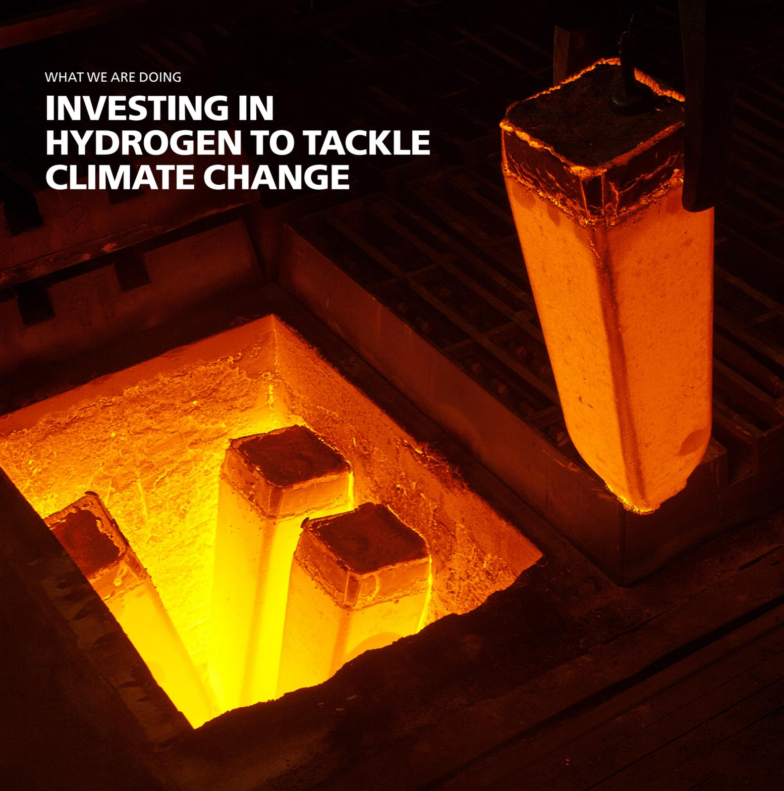
Hydrogen is not just a gas – it is an ingenious energy source that will play a key role in our efforts to achieve zero carbon emissions. We can produce it using electrolysis with 100% fossil-free electricity. When burned with oxygen, it emits nothing but water vapor and recoverable heat. Our plan is to switch our heating of steel prior to rolling, from fossil fuels to hydrogen – and a full-scale trial shows it works!
