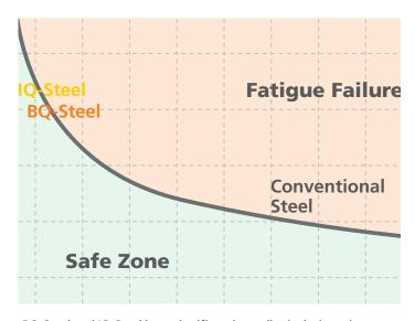
BQ-Steel and IQ-Steel have significantly smaller inclusions sizes compared to conventional steel. Note how the curve in the upper-left-hand corner is much steeper, meaning that the gain in fatigue strength is increasing exponentially.
