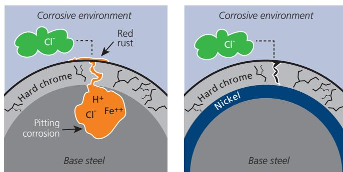
Corrosion mechanism of hard chrome plated bar
